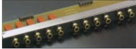
Hermetically sealed relays connected directly to gold-plated input/output jacks
